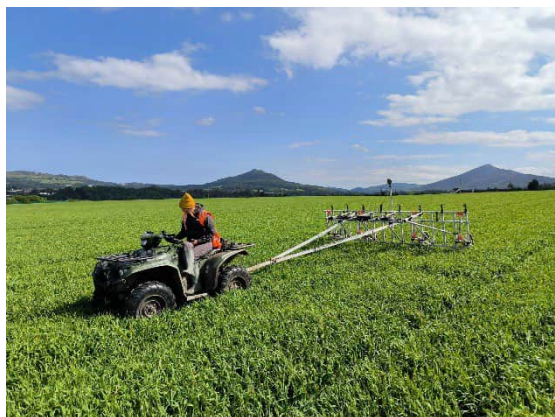
SENSYS MAGNETO MXV3 8-sensor fluxgate gradiometer cart system
