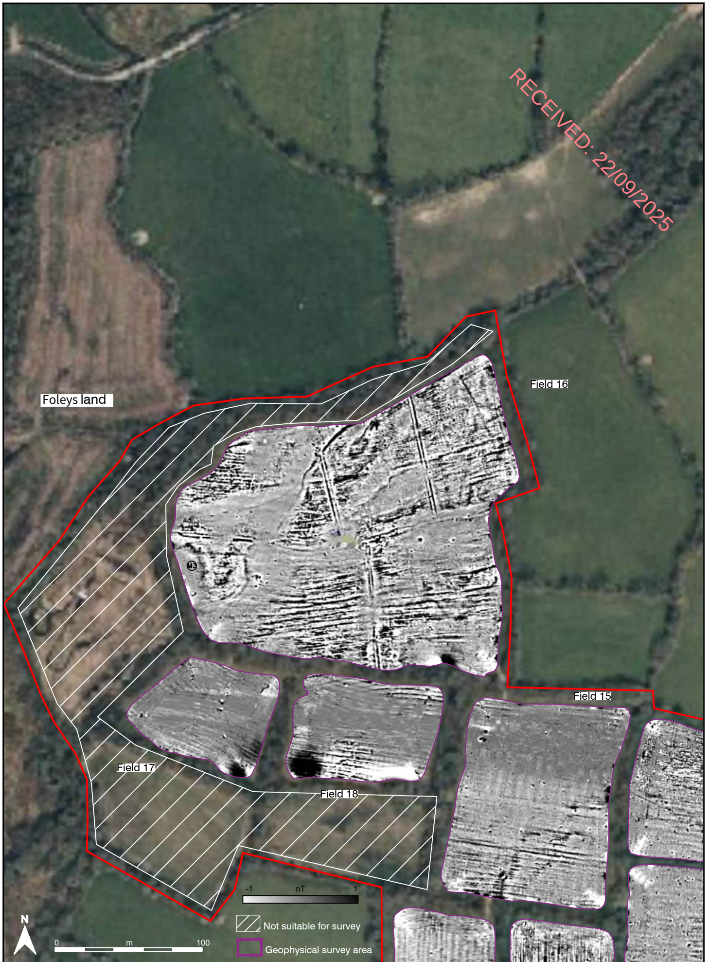
Figure 13 Aerial view of site, showing geophysical survey results for Foleys land (greyscale images) fields 15 to 18
