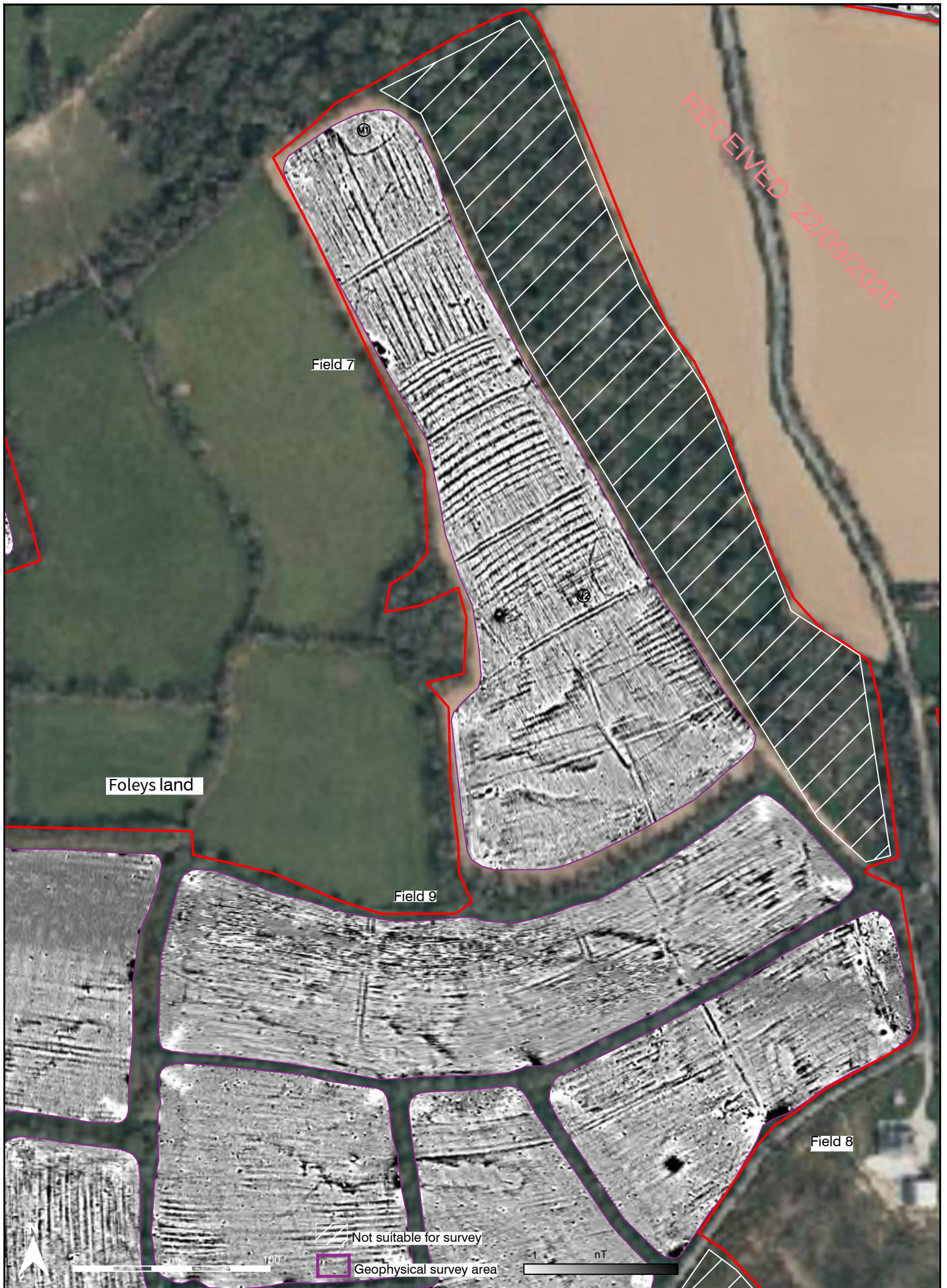
Figure 17 Aerial view of site, showing geophysical survey results for Foleys land (greyscale images) fields 7 to 9
