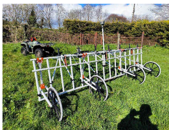
SENSYS MAGNETO MXV3 8-sensor fluxgate gradiometer cart system
